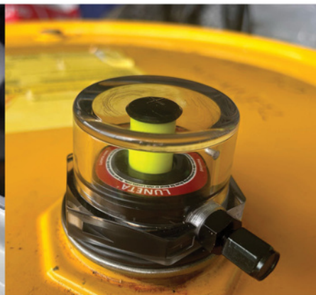
Air-Lock indicating good seal
