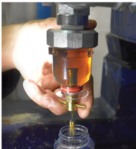
Sludge Pump - Using Bowl to Purge Water and Sediment
